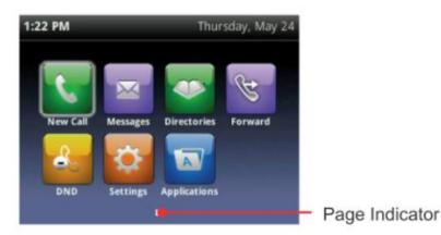
To change the displayed page, press the down or up arrow key. To change the highlighted entry, press the right or left arrow key. Press Select to access the desired menu.
